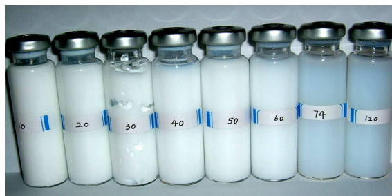
Fig. 1 Samples extracted from reaction system at different times for St and MMA surfactant-free emulsion polymerization in aqueous solution of PEG
